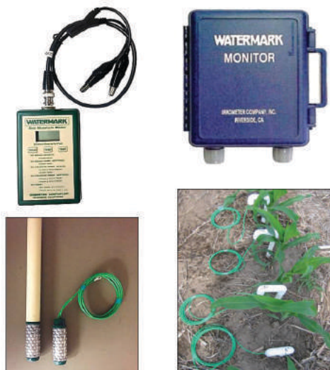
Figure 34. Watermark soil water monitoring system including sensors, hand-held readout and data logger.
